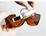
3. Straighten the telescope so that the eyepiece positions into the notch at the bottom of the slot.
