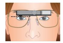
**C.** Adjust the bridge so the bottom of the eyepiece is positioned at the top of the pupil or the bottom of the upper lid – whichever is lower.
