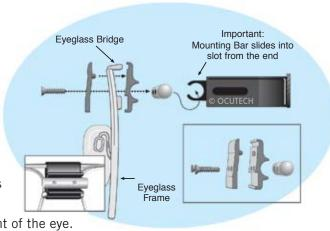
**IMPORTANT:** The telescope DOES NOT clip-off the frame. The frame mounting assembly provides a limited range of tilt angle. DO NOT force the angle beyond its free range of adjustment. THIS MAY DAMAGE the telescope and result in a repair.
